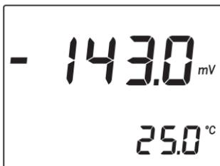
The "ATC" (or "MTC") tag is turned off because mV readings are not temperature compensated.
