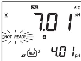
If you're going to calibrate with a different buffer, select the desired value by pressing the arrow keys.
