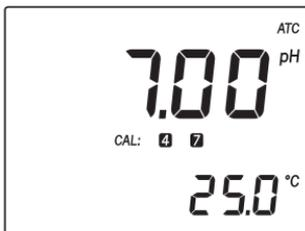
In order for the instrument to measure the pH accurately, temperature must be taken into consideration. If the sample temperature is different from the temperature at which the pH electrode was kept, allow a few minutes to reach thermal equilibrium.
