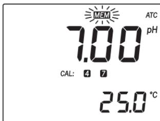
**Note:** While in MEM mode, the user can switch between pH and mV by pressing the RANGE key (**Mi 151** only).
