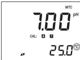
The "MTC" tag and up & down arrows symbols light up on the LCD to indicate that the instrument is in MTC mode and the arrow keys can be used to enter the desired temperature value.
